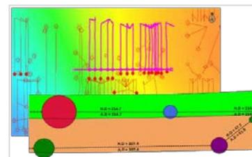
Absolute and horizontal distances between wells drilling inside the same target can be annotated very easily on the block diagram. Likewise, boundary distances between edge wells can also be annotated on the block diagram. Additionally, you can add formation thickness, distance filtering on the basis of formations and wellbore custom properties to get the complete picture of drilling wells and their placement inside the respective target formations.
